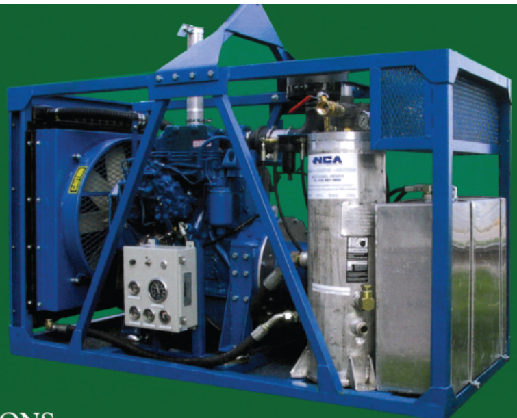
Bush Guard, Rigid Frame and Fuel Tank
