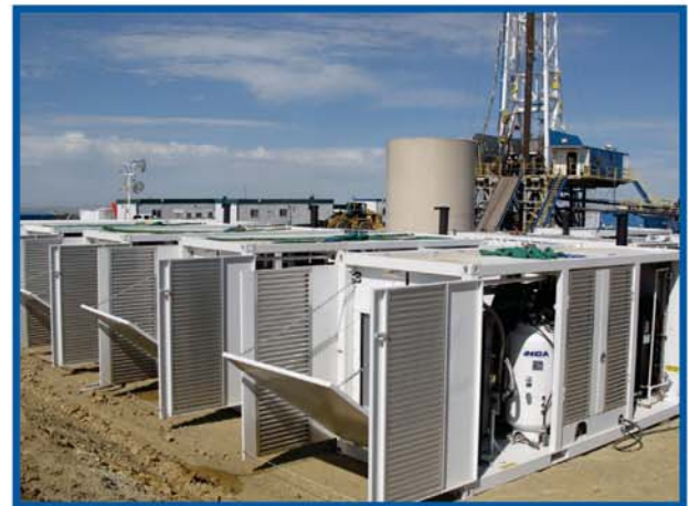
Containerized NCA Diesel Air Compressors with many client specific features
